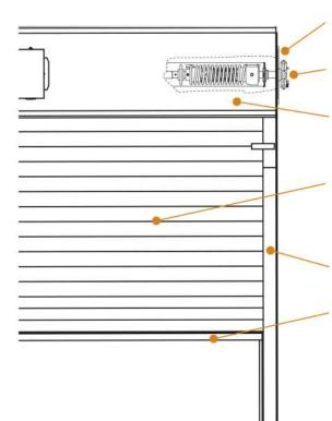
**BRACKETS** - Steel with powder coating to match curtin.
