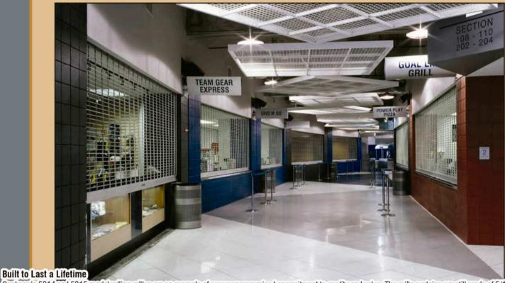
Cookson's 5014 and 5015 model rolling grilles are an example of our uncompromised commitment to quality and value. The grille curtains are still made of 5/16" solid aluminum rods rather than hollow rods used by other manufacturers. The links are 1/8" or 3/16' thick aluminum shapes rather than thinner gauge materials. The links are kept in position by composite tube spacers rather than inexpensive fasteners. The aluminum extruded guides and bottom bars are still made of heavy-walled shapes.
